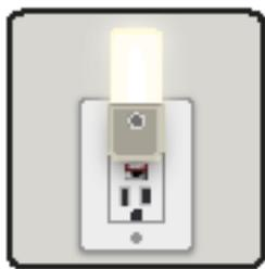
2. Plug an ordinary nightlight into the GFCI and turn it ON. The light should now be on.
