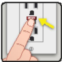
1. Push the "reset" button on the GFCI to prepare the outlet
