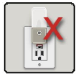
5. If the nightlight does not turn off when the "test" button is pushed, then the GFCI is not properly protecting you from shock or electrocution. Contact a licensed electrician to check the GFCI and correct the problem.
