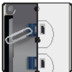
Though they look like standard outlets, TRRs have a built-in shutter system that prevents the insertion of foreign objects.
