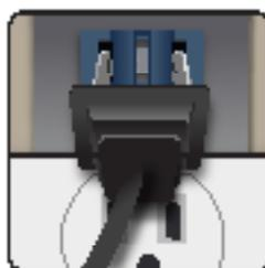
Plugs can still be easily inserted when equal pressure is applied to both slots.
