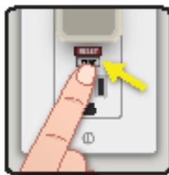
3. Push the "test" button of the GFCI. The nightlight should turn OFF.
