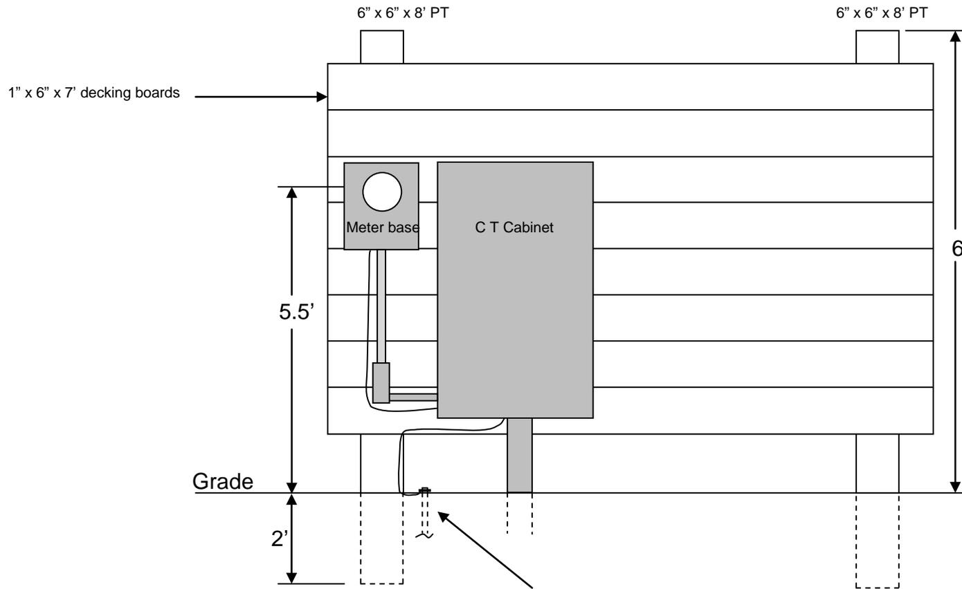
8' ground rod, clamp and #6 bare copper ground wire
